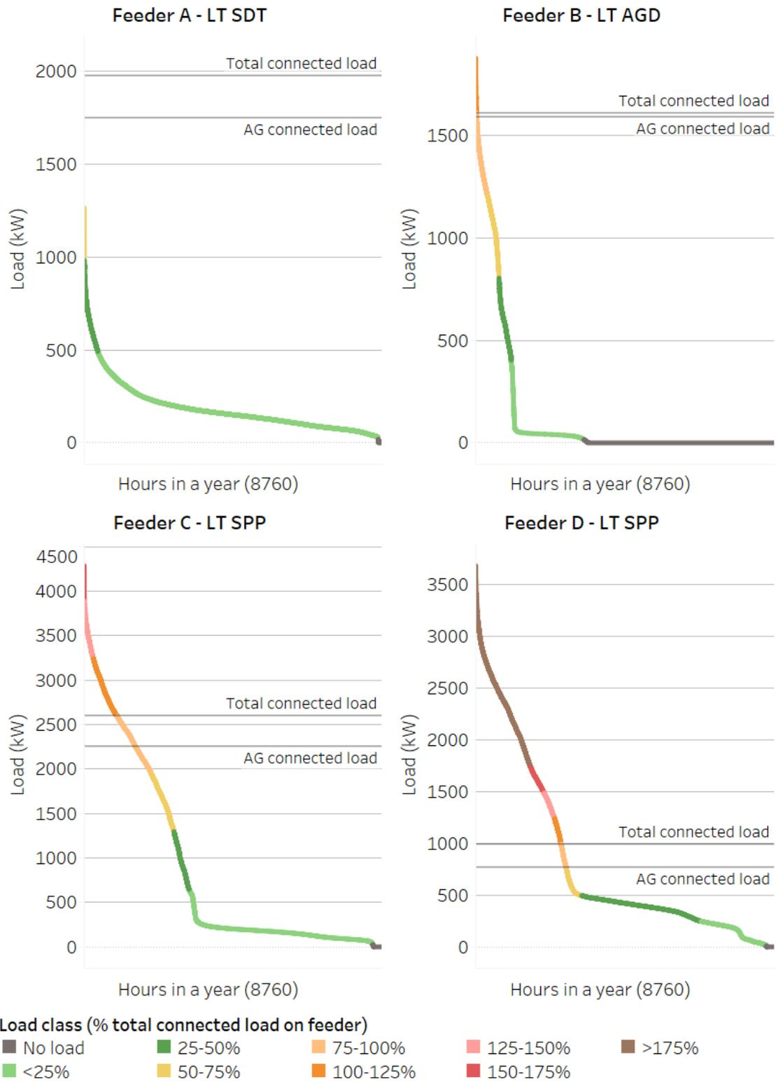
Figure 5.2 Feeder loading profiles- Feeder Current Duration Curves
