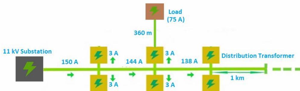
All the DTs are assumed to be equally loaded and receive the same input at the H.T. side, which equals feeder input less annual feeder losses divided by total number of DTs. Losses in DTs are worked out after taking into account the DT efficiency of 98%.
