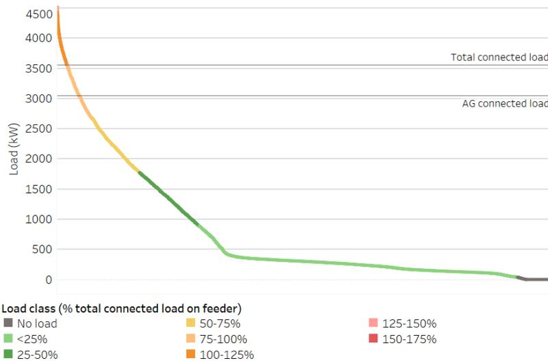
For the purpose of analysis, a feeder network has been divided into three elements: 1. Feeder line 2. Distribution transformers 3. Low voltage (440 V) circuit. Annual technical losses are arrived at after adding losses in each of these three elements for all loading classes i.e. from excess load to very-low load condition.
