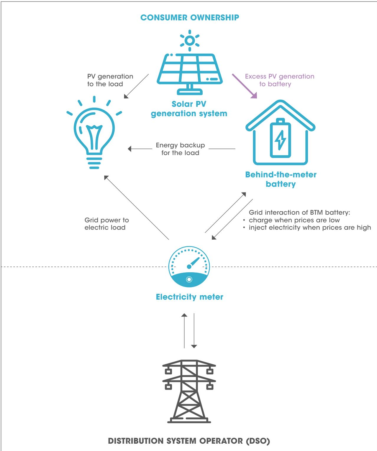
A BTM battery installed at the consumer’s premises can store electricity that either is produced from on-site solar rooftop PV systems (if applicable) or is drawn from the distribution grid, generally when electricity prices are low. This stored electricity can then be used to meet the consumer’s electricity needs, or it can be injected back into the distribution grid when electricity prices are high.
