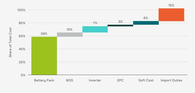
1 MW / 4 MWh Battery System
