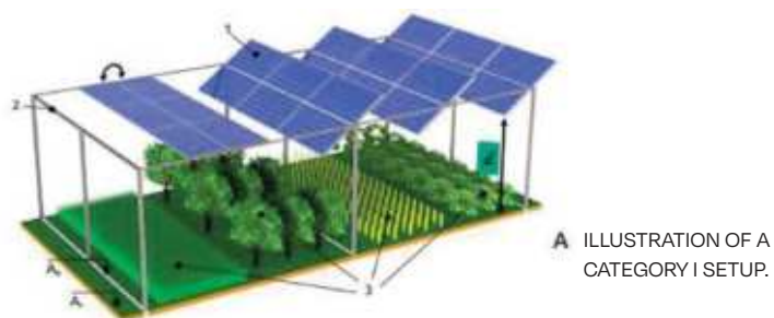
FIGURE 4 DIFFERENT TYPES OF AGRIPV INSTALLATIONS
