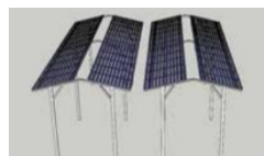
Overhead East-West Configuration
